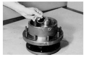
**NOTE:** Make sure retaining ring is securely seated in groove.
