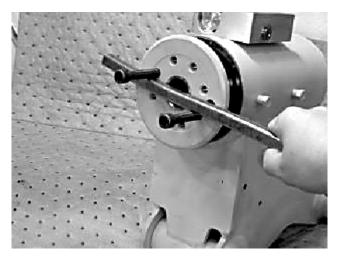
**13.** Install stop tube on shaft end. Stop tube is an available option to limit rotation of an actuator.
