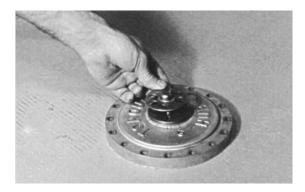
8. Place two remaining bolts (6C) in bolt holes in disconnect cap (6D). Tighten bolts.
