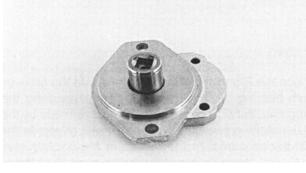
1. Install new shaft seal in mounting flange with part lumber side facing outboard. Press the seal into the seal lore until the seal reaches the bottom of the bore. Uniform pressure must be used to prevent misalignment or damage to the seal.
