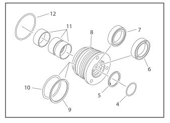
Figure 5-17. Cylinder Head Disassembly
