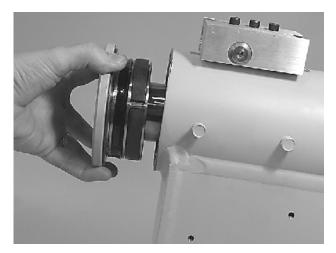
**11.** Looking from view shown, use existing timing marks to line up gear teeth on shaft (2) with gear teeth on inside of piston (3). Tap flange end of shaft with a rubber mallet until gear teeth engage.
