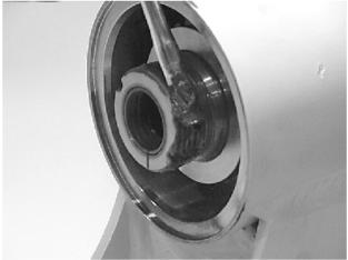
15. Install 0-ring (204) and back-up ring (207) into inner seal groove on end cap (4).
