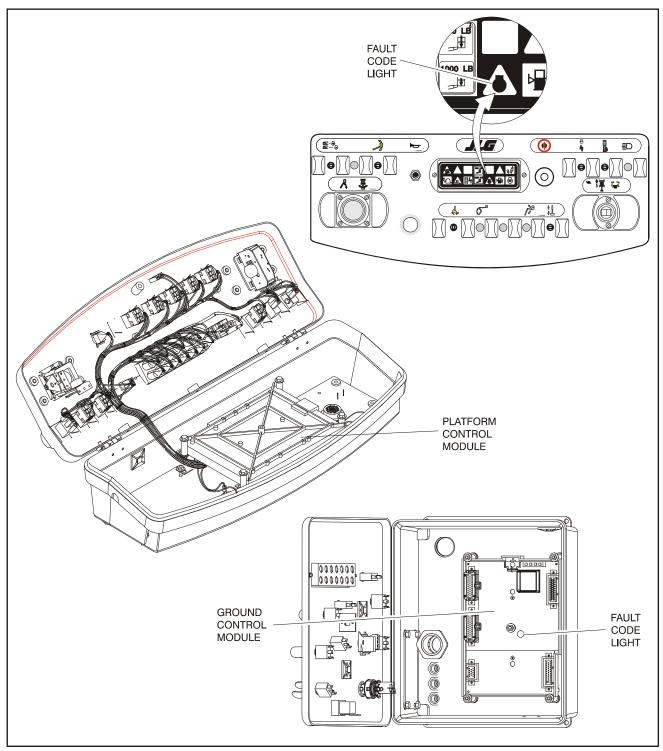
Figure 6-3. Control Module Location
