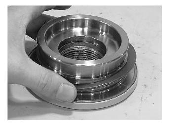
**18.** Remove wiper seal (304.1) from groove in end cap (4) and shaft (2).
