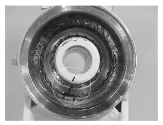
**12.** Install two bolts in threaded holes of flange. Using a bar, rotate shaft clockwise until wear guides are seated in housing bore.
