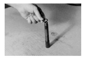
5. Place one spring (7C) on smooth end of input shaft (7A).
