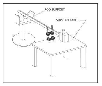
Figure 5-73. Cylinder Rod Support
