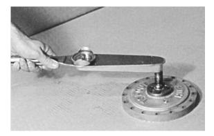
10. Apply a light coat of "Never-Seize" to pipe plug (6H) and tighten it in pipe plug hole in cover (6A).
