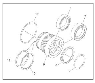
Figure 5-76. Cylinder Head Disassembly
