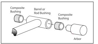
Figure 5-57. Composite Bushing Installation
