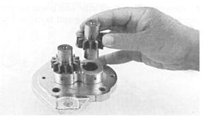
**11.** Remove idler shaft from bearing block.
