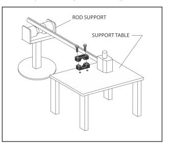
Figure 5-14. Cylinder Rod Support
