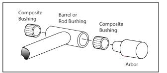
Figure 5-28. Composite Bushing Installation
