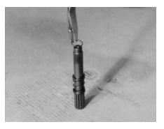
8. With large splined end down, place input shaft subassembly (7) in spindle (1A).
