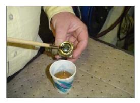
**3.** Turn fitting over and repeat previous step to O-ring on other side of fitting. Make sure entire O-ring is coated with hydraulic oil.
