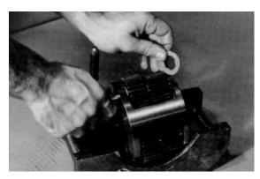
8. Use an alignment punch or similar tool to align roll pin holes in carrier housing (3A) and planet shaft (3E).
