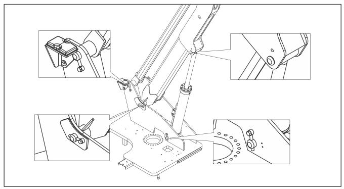
Figure 4-1. Location of Components - Boom Removal
