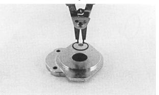
**14.** Turn the mounting flange over, with the shaft seal up, and remove the retaining ring with proper snap ring pliers.
