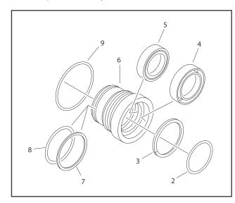
Figure 5-67. Cylinder Head Assembly
