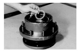
4. Stand input shaft (7A) on its splined end. Place one spacer (7D) on smooth end of input shaft (7A).
