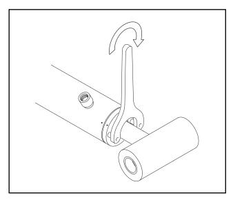
Figure 5-31. Cylinder Head Installation
