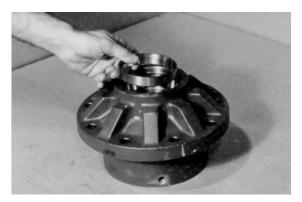
2. Press nine studs (1N) in stud holes in hub (1G).
