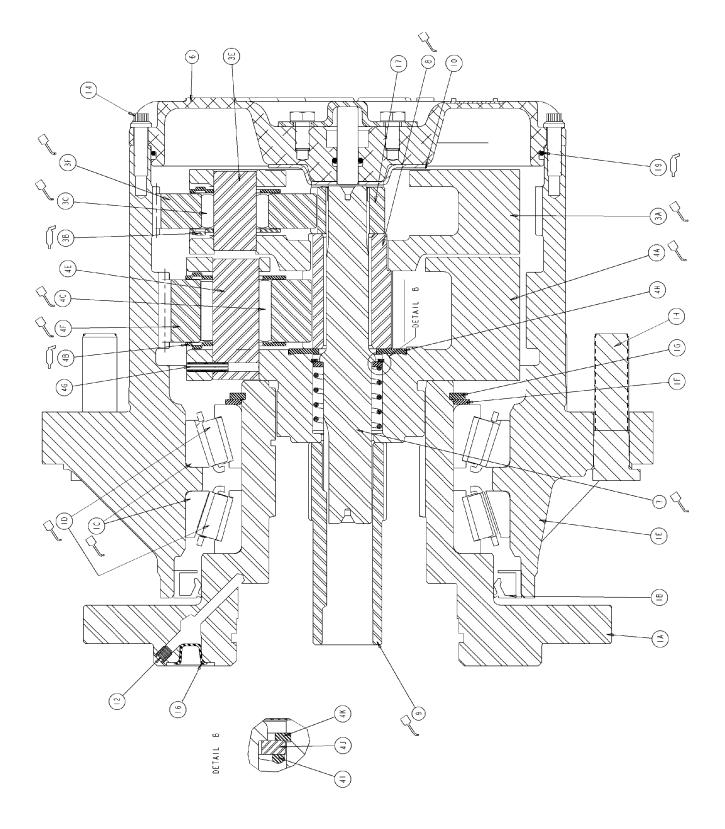
Figure 3-13. Assembly Drawing - Without Integral Input Brake - Sheet 1 of 2
