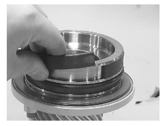
**16.** To remove main pressure seals (205), cut them using a sharp razor blade. Do not to damage the seal groove.
