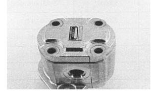
**15.** Install the two remaining dowel pins in the rear of the gear housing, if applicable, and place the end cover over the back of the pump.
