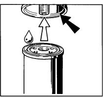
6. Manually screw in the new filter until the gasket is flush.
