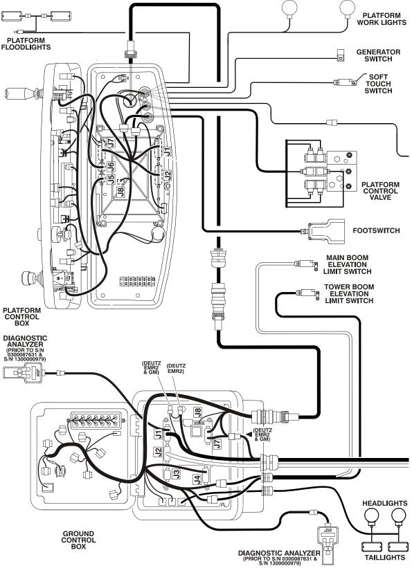
Figure 7-18. Electrical Components Installation - Sheet 1
