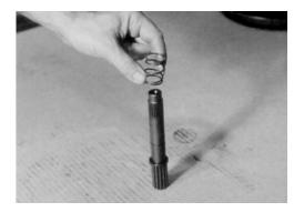
6. Place spacer (7D) on smooth end of input shaft (7A).
