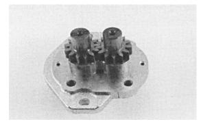
**9.** Install the idler gear shaft in the remaining position in the bearing block. Apply a light coat of clean oil to the face of the drive and idler gears.
