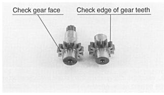
**4.** Inspect gear face for scoring or excessive wear. If the face edge of gear teeth are sharp, they will mill into the bearing blocks. If wear has occurred, the parts are unusable.
