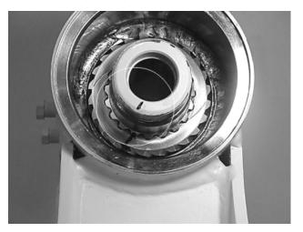
**10.** Remove shaft (2). It may be necessary to strike the threaded end of shaft with a rubber mallet.
