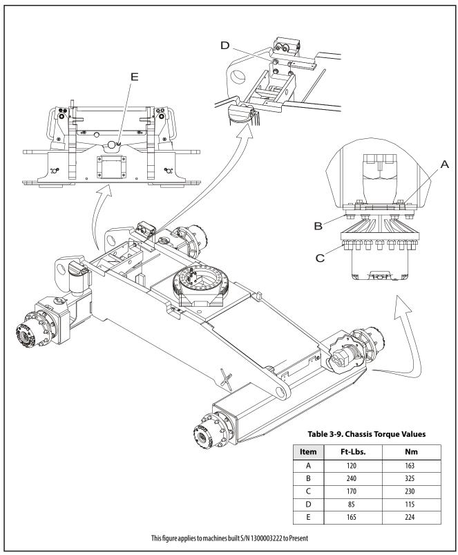
Figure 3-47. Chassis Torque Values - Sheet 2 of 2
