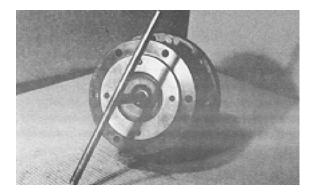
24. Leak test unit at a pressure of 5 psi for 2 to 3 minutes.
