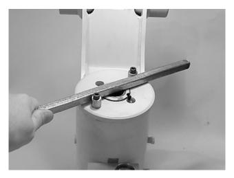
6. Remove end cap (4) and set aside for later inspection.
