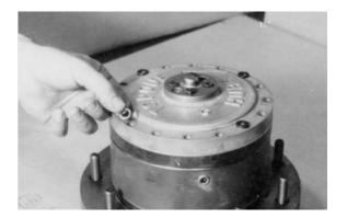
18. Place shoulder bolts (13) in four shoulder bolt holes in cover (6). Tighten by hand.
