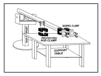
Figure 5-61. Cylinder Barrel Support
