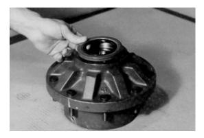
7. Oil spindle, then lower hub (1G), small end down, onto spindle (1A).
