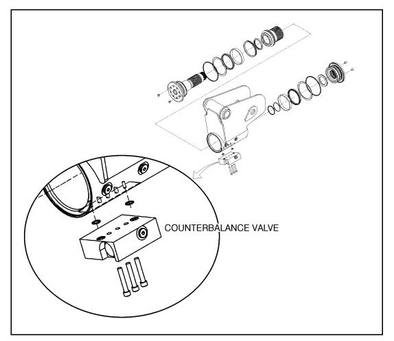
Figure 4-8. Rotator Counterbalance Valve
