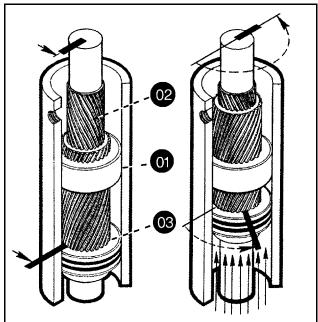
Bars indicate starting positions of piston and shaft. Arrows indicate direction they will rotate. The housing with integral ring gear remains stationary.
