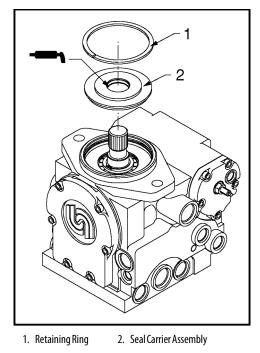
Figure 5-85. Shaft Seal Components
