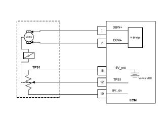
Electronic Throttle Actuator w/Analog Position Feedback
