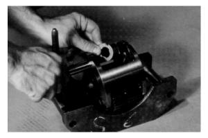
6. Following thrust washer, place cluster gear (3F), large end toward roll pin hole in carrier housing, on planet shaft (3E).
