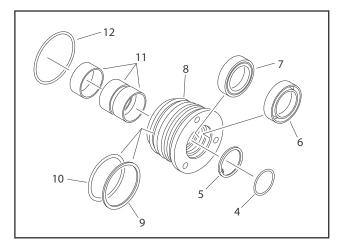
Figure 5-19. Cylinder Head Assembly
