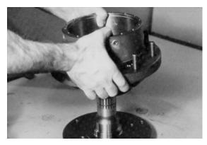
8. Press bearing cone (1F) on spindle (1A) in hub (1G).
