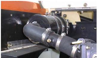
Lube Point(s) - Replaceable Element Interval - Every 6 months or 300 hours of operation or as indicated by the condition indicator
