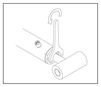
Figure 5-33. Cylinder Head Removal
