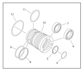
Figure 5-56. Cylinder Head Disassembly
