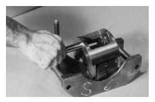
5. Place one thrust washer (3B) onto the end of planet shaft (3E) inside carrier. Fit tang of thrust washer into the slot on the inside edge of the planet shaft hole.
