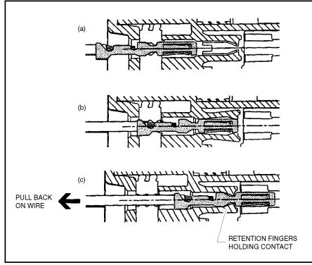
Figure 7-7. Connector Assembly Figure 2
