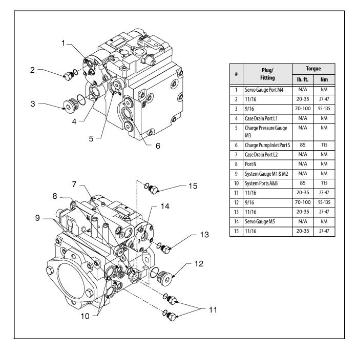
Figure 5-83. Plugs/Fittings Size & Torque
