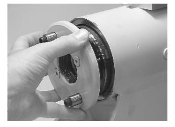
17. Tighten end cap (4). In most cases original holes for lock pins line up.
