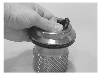
Beginning with inner seal (200) insert one end of backup ring in lower groove and feed the rest in using a circular motion. Make sure wedged ends overlap correctly.
