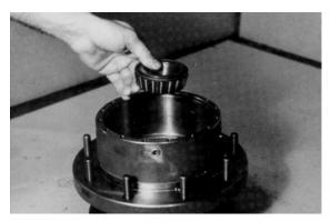
9. Place spacer (1H) on spindle (1A) in hub (1G).
