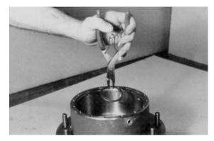
11. At this point hub-spindle sub-assembly is complete.
