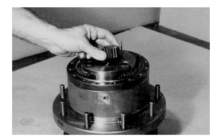
14. Oil all exposed surfaces inside hub (1G). Place thrust washer (11) in counterbore in top of carrier.
