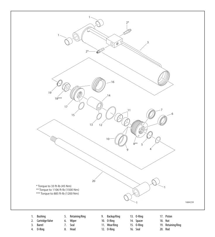
Figure 5-5. Tower Lift Cylinder
