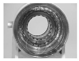
**10.** Install shaft (2) in piston (3). Dol not damage seals. Do not engage piston gear teeth yet.
