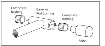
Figure 5-47. Composite Bushing Installation
