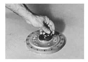
6. Using a torque wrench, apply 36 to 49 in-lb (4 to 5 Nm) of torque to both bolts (6C).
