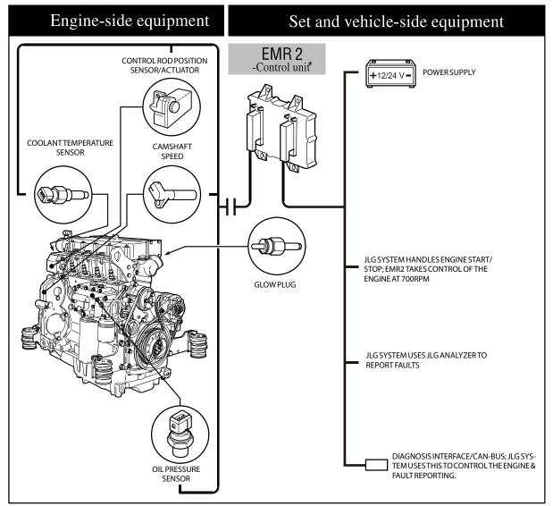
Figure 3-56. EMR 2 Engine Side Equipment
