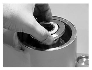
**8.** Every actuator has timing marks for proper engagement.
