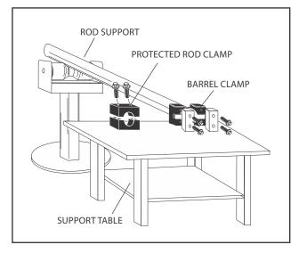
Figure 5-2. Cylinder Barrel Support
