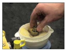
**3.** After lifting fitting, a small droplet should form and drip from bottom of fitting. This indicates an even coating of oil.
