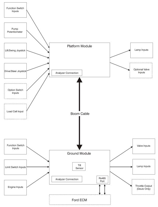
Figure 6-4. ADE Control System Block Diagram
