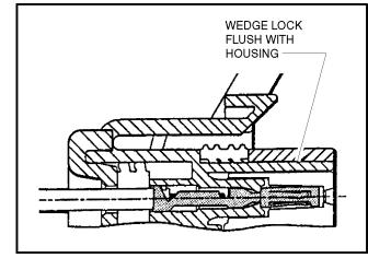
Figure 7-9. Connector Assembly Figure 4
