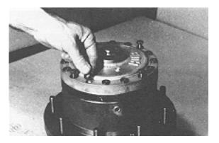
20. Place 12 bolts in remaining bolt holes in cover (6) and tighten.
