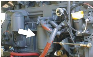
Lube Point(s) - Replaceable Element Interval - Every Year or 600 hours of operation
