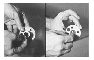
2. Place O-ring (6G) on cover cap (6B) so that it rests against flange of cover cap.
