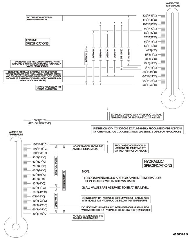
Figure 2-2. Engine Operating Temperature Specifications - Perkins
