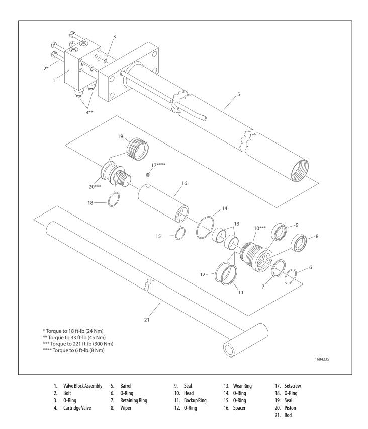
Figure 5-35. Telescope Cylinder
