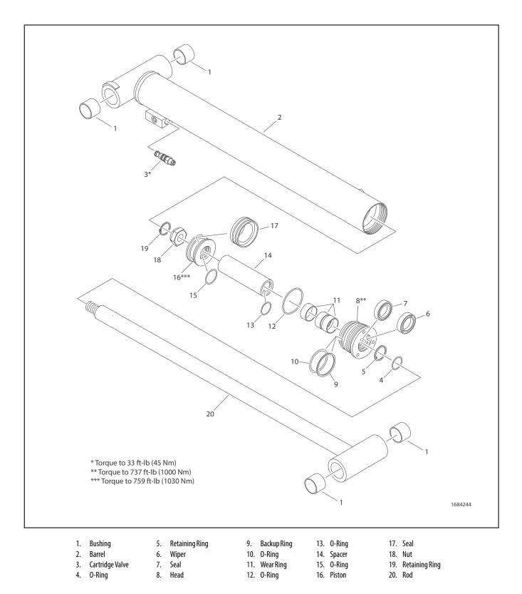
Figure 5-15. Main Lift Cylinder
