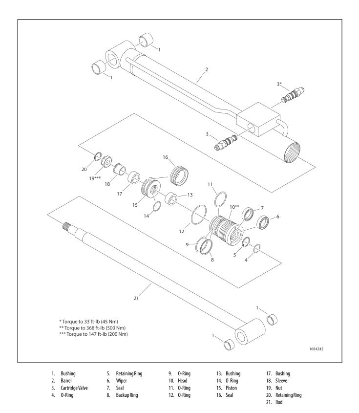
Figure 5-54. Jib Lift Cylinder
