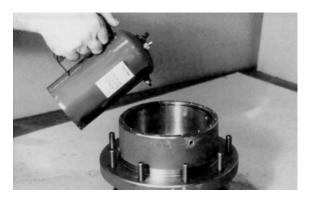
Place internal gear (2) in hub (1G) so its internal splines mesh with external splines of spindle (1A). Oil internal gear (2).
