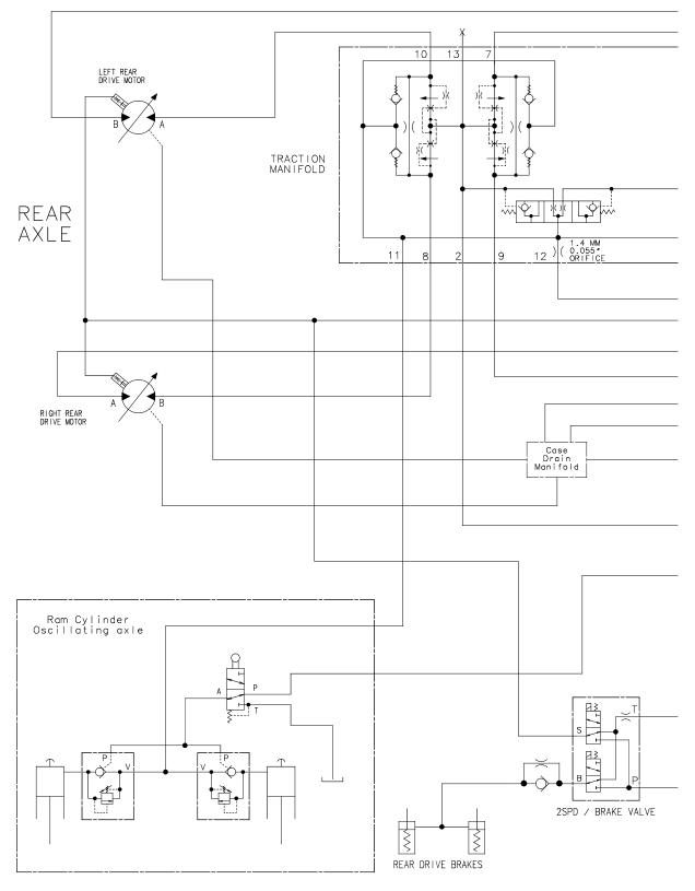
Figure 5-94. Hydraulic Schematic - Sheet 5 of 6
