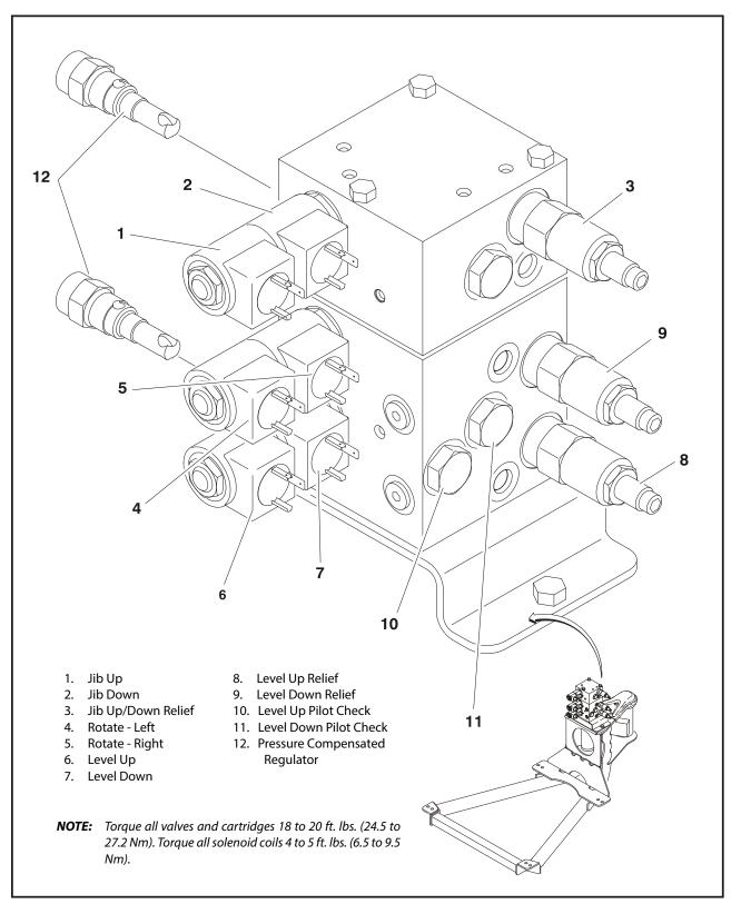
Figure 5-91. Platform Control Valve
