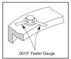
Figure 3-50. Swing Bearing Feeler Gauge Check
