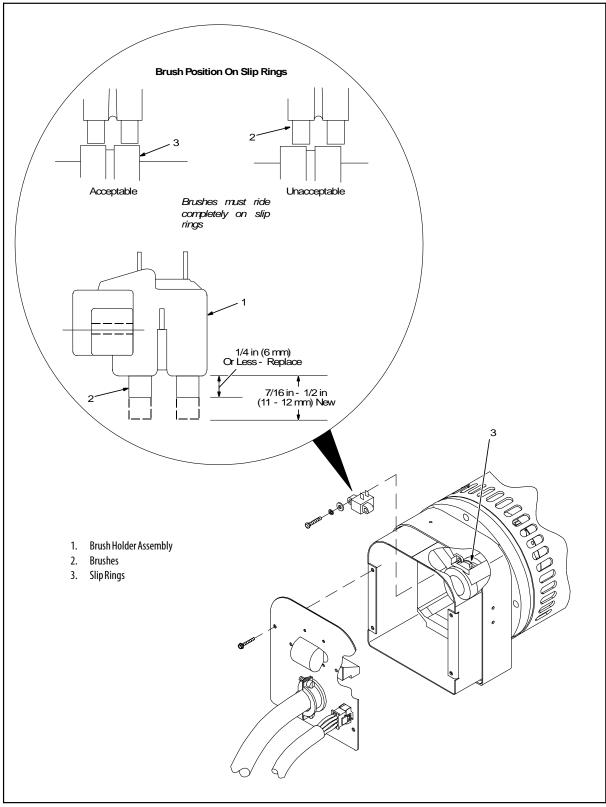
Figure 3-54. Inspecting Generator Brushes, Replacing Brushes, and Cleaning Slip Rings
