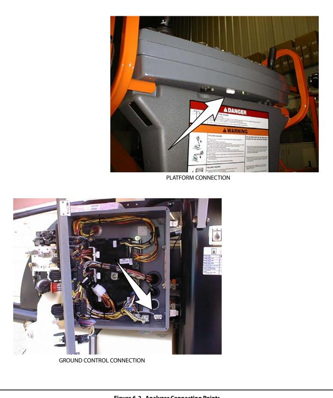
Figure 6-2. Analyzer Connecting Points
