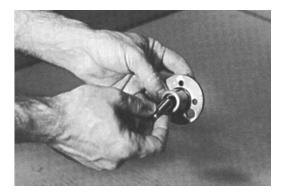
4. Set cover (6A) on table, exterior side up. Place cover cap (6B) on cover (6A), aligning pipe plug hole in cover cap over pipe plug hole in cover.
