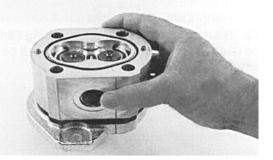
**9.** Carefully remove gear housing and place on work bench. Make sure the rear bearing block remains on the drive and idler shafts.
