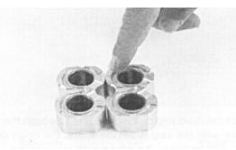
**3.** Place front and back bearing blocks on a clean surface with the E-seal grooves facing up. Apply a light coating of petroleum jelly in the grooves. Also coat the E-seal and backup with the petroleum jelly, this will help keep the seals in place during reassembly.
