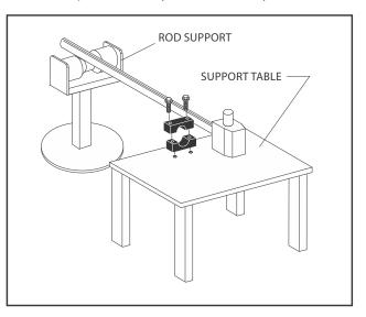
Figure 5-4. Cylinder Rod Support
