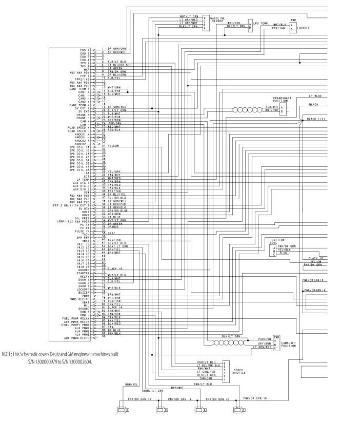
Figure 7-28. Electrical Schematic - Deutz EMR2 & GM Engine - Sheet 5 of 6
