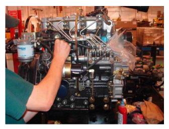
2. With control linkage pushed against idle stop, begin to make adjustments to actuator linkage to align bearing of spherical rod end with control linkage bolt hole. When making linkage adjustments, thread spherical rod end and threaded rod evenly (for every turn of spherical rod end, turn threaded rod.)
