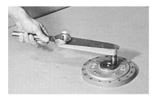
7. With large end down, place disconnect cap (6D) on cover cap (6B), aligning pipe plug hole in disconnect cap over pipe plug hole in cover cap.
