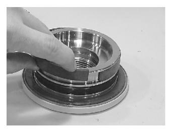
**6.** Install inner T-seal (200) in piston (3) using a circular motion.
