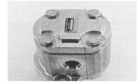
**16.** Install the four spacers, if applicable, and hex head bolts through the bolt holes in the end cover, hand tighten.
