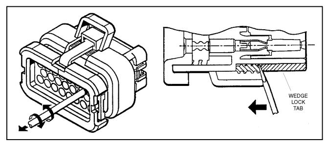
Figure 7-10. Connector Disassembly
