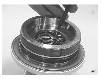
**15.** Remove wear guides (302) from end cap (4) and shaft (2).
