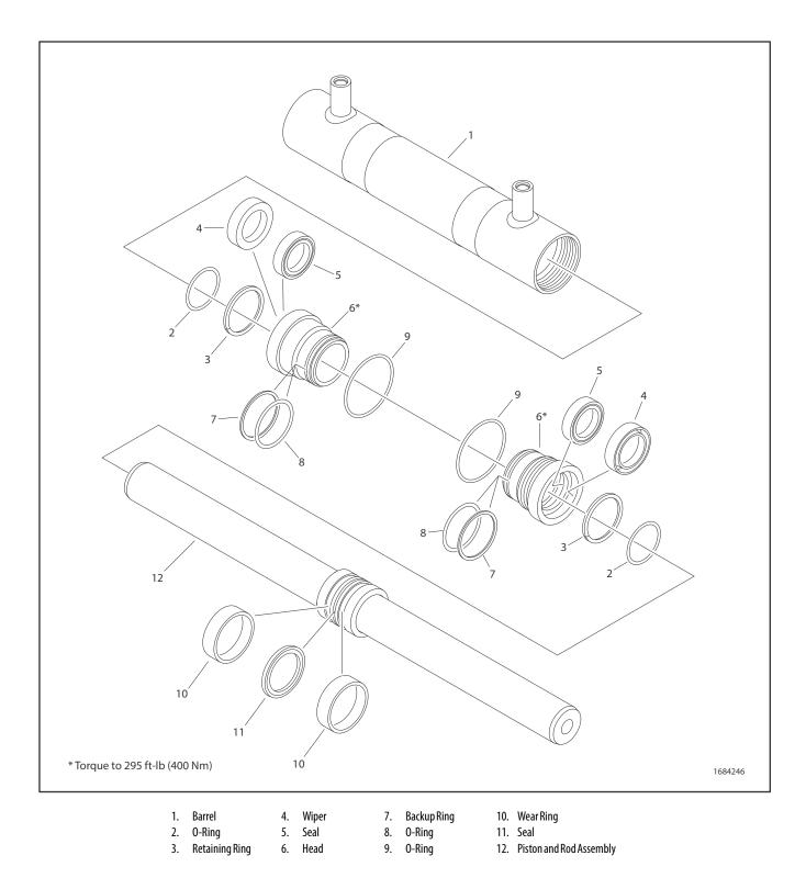
Figure 5-64. Steer Cylinder Assembly
