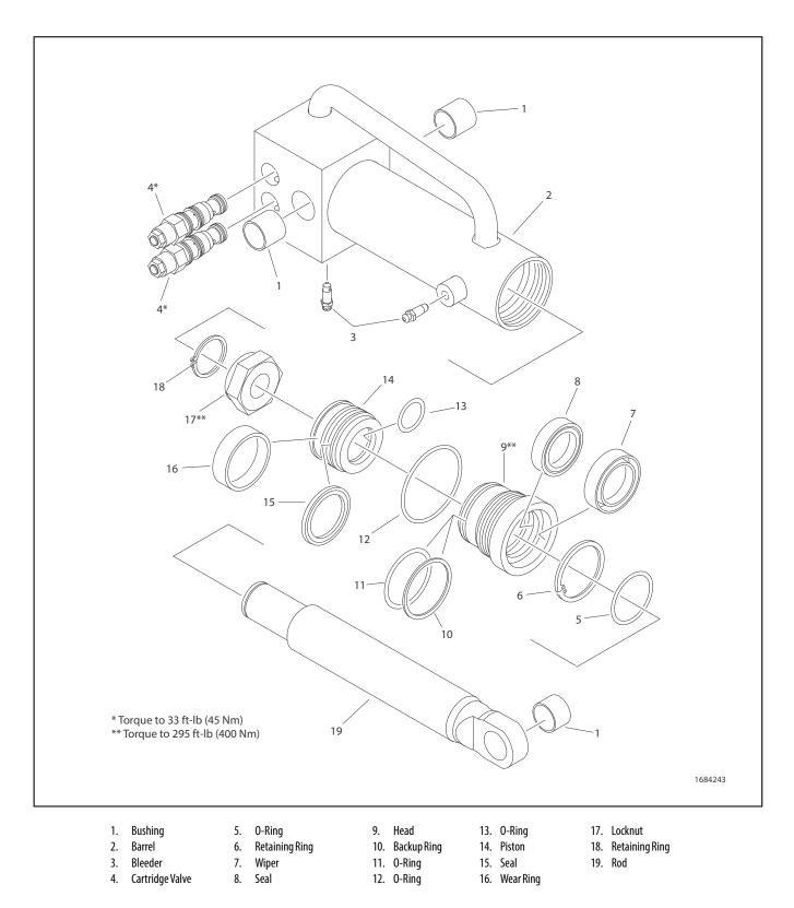
Figure 5-74. Axle Lockout Cylinder (Inside Frame)
