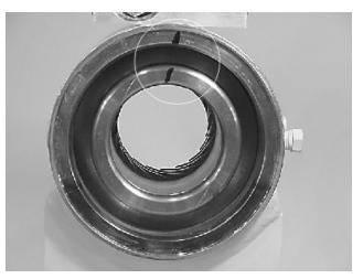
**9.** Looking from opposite end of housing (1) you can see if timing marks line up. When they do, tap piston (3) in until gear teeth mesh together. Tap piston in housing until it bottoms out.
