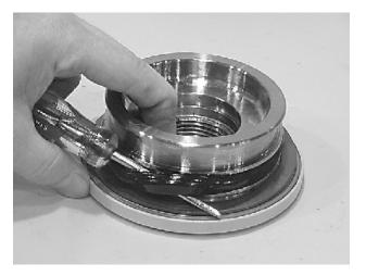
5. Install wear guide (302) on end cap (4) and shaft (2).
