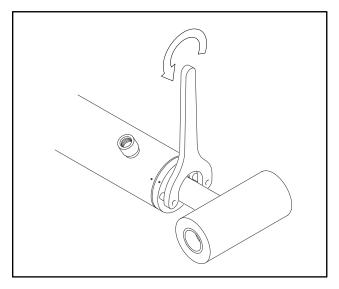
Figure 5-42. Cylinder Head Removal
