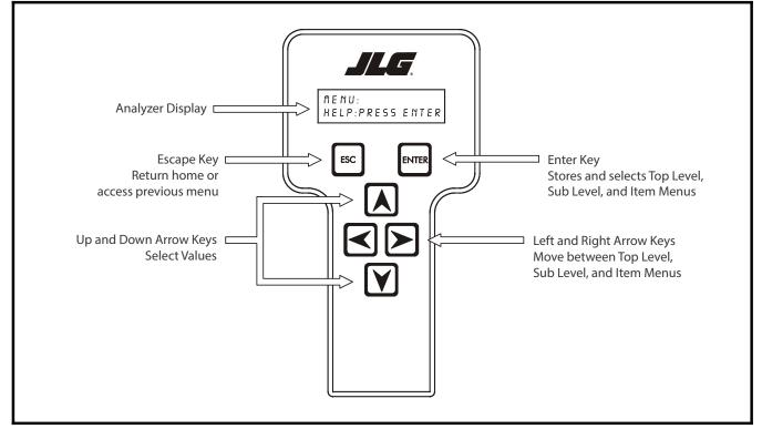
Figure 6-1. Hand-Held Analyzer (WANALYZER Controls and Display Similar)
