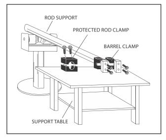
Figure 5-12. Cylinder Barrel Support
