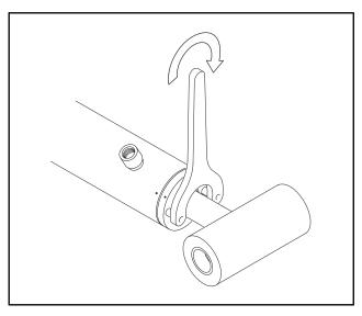
Figure 5-21. Cylinder Head Installation
