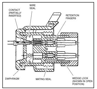
Figure 7-5. Connector Assembly Figure 1
