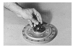
9. Using a torque wrench, apply 36 to 49 in-lb (4 to 5 Nm) of torque to both bolts (6C).
