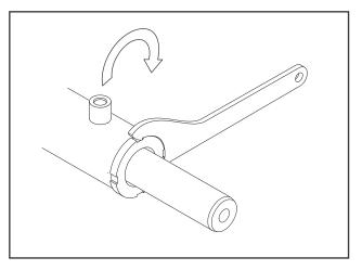
Figure 5-69. Cylinder Head Installation
