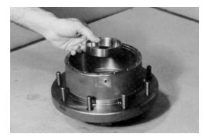
5. Set hub (1G) on its large end. Place bearing cone (1D) in bearing cup (1C).
