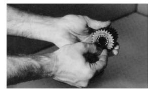
4. Set carrier housing (3A) on table, sideways. Insert a planet shaft (3E), roll pin hole last, in one of planet shaft holes from roll-pin-holed side of carrier housing (3A).
