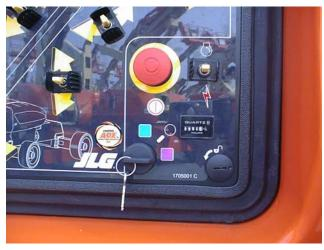
2. Plug the analyzer into the connector inside the Ground control box.
