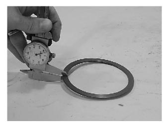
**3.** Inspect wear guide condition and measure thickness (not less than 0.123" or 3.12 mm).
