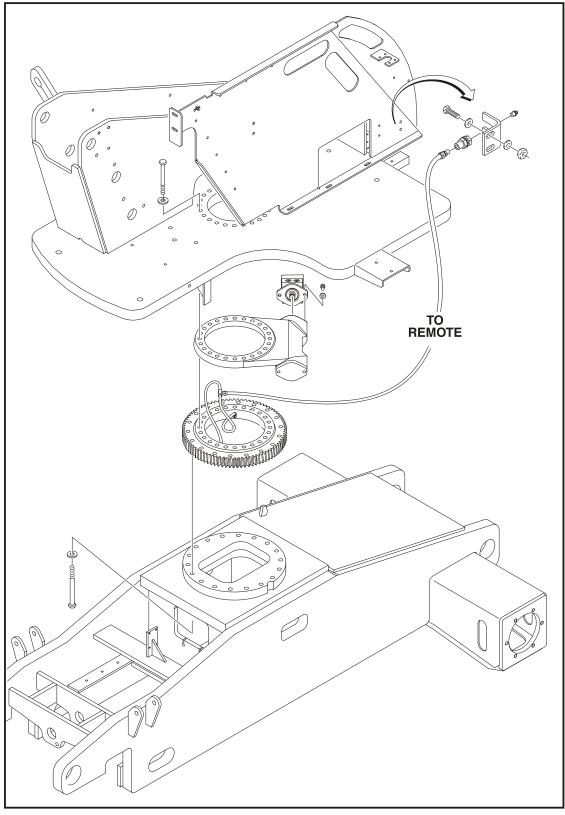
Figure 3-48. Swing Bearing Installation
