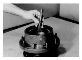
9. Place thrust spacer (9) on input shaft (7).
