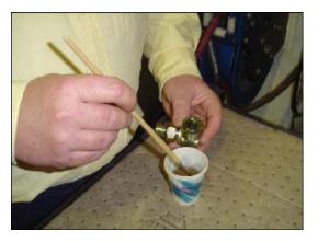
**2.** Hold fitting over hydraulic oil container and brush an even film of oil around entire O-ring in fitting. Make sure O-ring is completely saturated.
