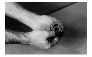
3. Line remaining half of cluster gear (3F) with 16 needle rollers.
