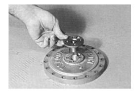
5. Place two cover cap bolts (6C) in any two bolt hoes that are 180° apart on cover cap (6B) and tighten bolts.
