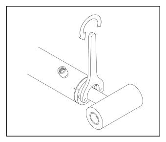
Figure 5-3. Cylinder Head Removal
