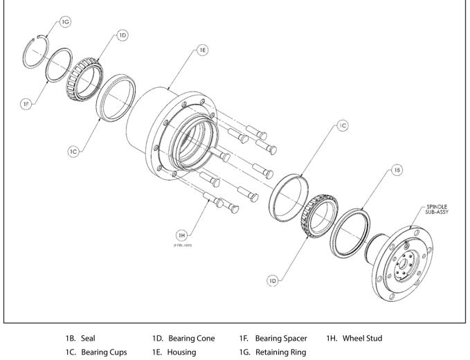
Figure 3-5. Housing-Spindle Disassembly
