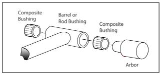
Figure 5-8. Composite Bushing Installation
