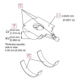
Inspect the journal bearings for damage or excessive wear. Replace journal bearings if scratched, warped, or excessively worn. The polymer wear layer must be smooth and intact.
