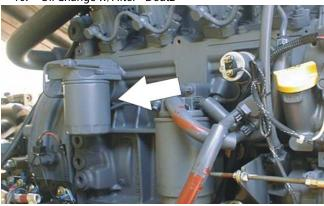
Lube Point(s) - Fill Cap/Spin-on Element Capacity - 11 Quarts(10.5 L) Crankcase; 5 Quarts (4.7 L) Cooler Lube - EO Interval - Every Year or 1200 hours of operation Comments - Check level daily/Change in accordance with engine manual.
