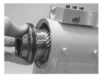
8. Looking from angle shown, rotate piston (3) until marks on piston and housing (1) made during disassembly line up as shown. Using a rubber mallet, tap piston into housing up to the point where gear teeth meet.
