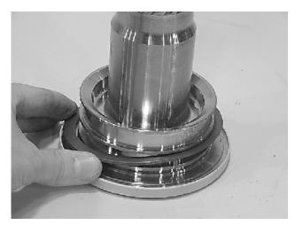
Install wiper seal (304.1/green 0-ring) in groove on shaft
