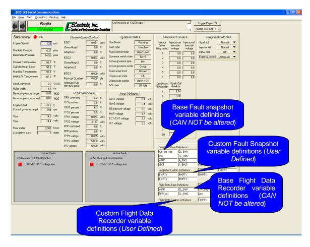
Figure 3-71. Faults Page with Active Fault Message
