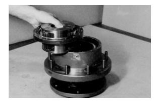
13. With internal splines facing up (counterbore end facing down), place input gear (8) into mesh with carrier subassembly (3).
