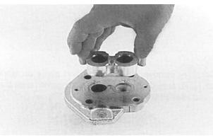
**13.** Remove the front bearing block.
