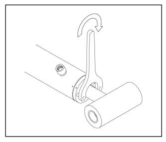
Figure 5-11. Cylinder Head Installation
