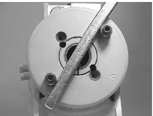
Place lock pins (109) provided in Helac seal kit in holes with dimple side up. Using a punch, tap lock pins to bot-
