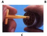
Figure 7-16. HD/HDP Contact Removal
