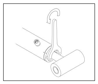
Figure 5-13. Cylinder Head Removal
