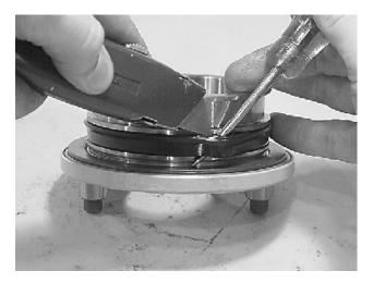
17. Remove thrust washers (304), from end cap (4) and shaft (2).
