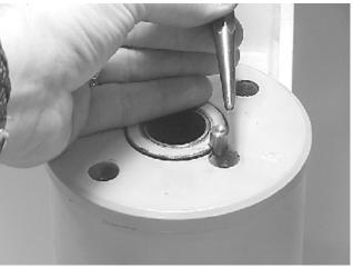
Insert set screws (113) over lock pins. Tighten to 25 in-lb 19. (2.8 Nm).
