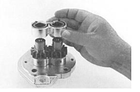
**10.** Remove rear bearing block from drive and idler shafts.
