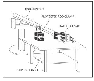
Figure 5-32. Cylinder Barrel Support
