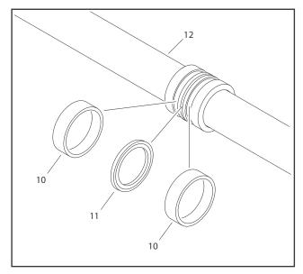
Figure 5-65. Piston Seal and Wear Ring
