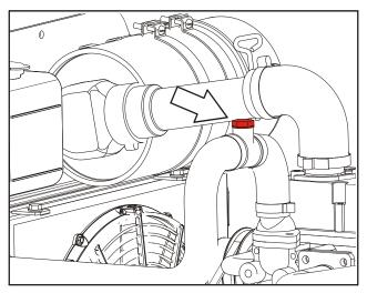
**5.** Using sealant JLG P/N 0100020 (Loctite #567), install plug back into the adapter.
