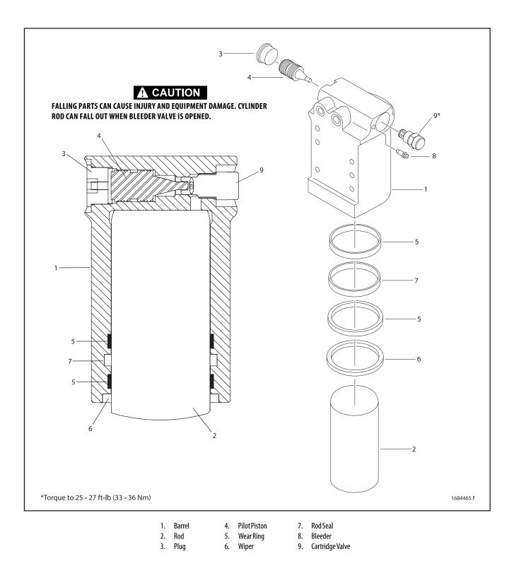
Figure 5-70. Axle Lockout Cylinder
