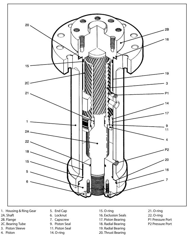
Figure 4-5. Rotator Assembly - Cutaway
