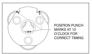
Figure 3-23. Cluster Gear Punch Marks
