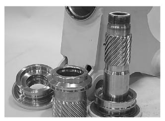
**2.** Inspect thrust washers (304) for rough or worn edges and surfaces. Measure thickness to make sure it is within specifications (Not less than 0.092" or 2.34 mm).
