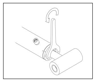
Figure 5-23. Cylinder Head Removal
