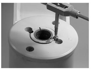
If pin will not come out with "Easy Out", use 5/1 6" drill bit to a depth of 1/2" (12.7mm) to drill out entire pin.
