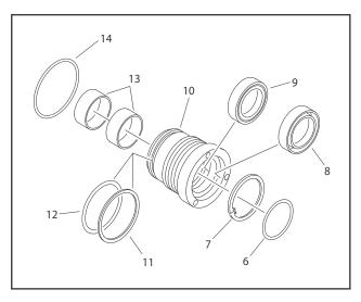
Figure 5-37. Cylinder Head Disassembly
