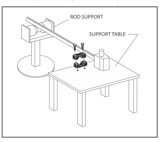
Figure 5-43. Cylinder Rod Support
