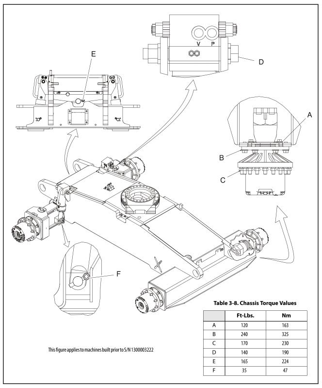
Figure 3-47. Chassis Torque Values - Sheet 1 of 2
