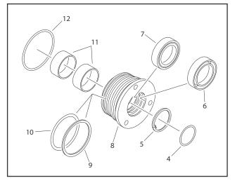
Figure 5-7. Cylinder Head Disassembly
