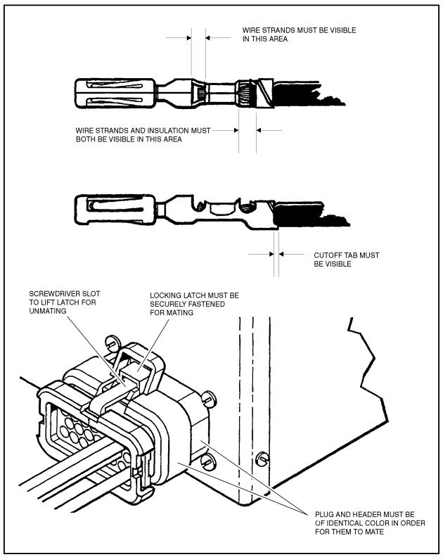
Figure 7-11. Connector Installation
