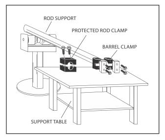
Figure 5-22. Cylinder Barrel Support
