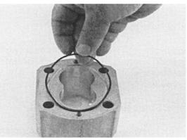
**12.** To install the O-rings in the gear housing, apply a light coating of petroleum jelly in the grooves on both sides of the gear housing. Also coat the new O-rings and install them in the grooves.
