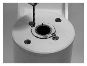
3. Remove lock pins using an "Easy Out" (Size #2 is shown).
