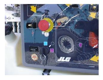
2. Plug analyzer in connector at base of platform control box.
