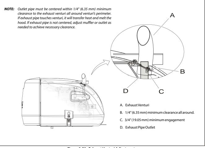
Figure 3-78. Exhaust Venturi Adjustment
