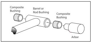
Figure 5-18. Composite Bushing Installation
