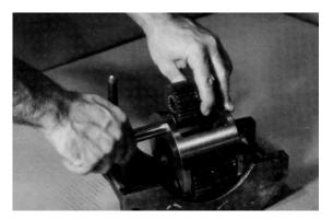
Following cluster gear, place one more thrust washer (3B) on planet shaft (3E) through opposite planet shaft hole in carrier housing (3A). 9. Drive roll pin (3G) down in aligned roll pin holes in carrier housing (3A) and planet shaft (3E).
