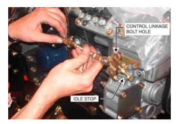
3. Once the adjustments have been made to align the spherical rod end bearing with the control linkage bolt hole, lengthen the actuator linkage by continuing to turn the spherical rod end and threaded rod 2-2 ½ turns (1-1 ¼ turns of spherical rod end and 1-1 ¼ turns of threaded rod.) This will provide 1/8" (3 mm) preload.
