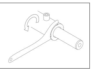
Figure 5-62. Removing Cylinder Head
