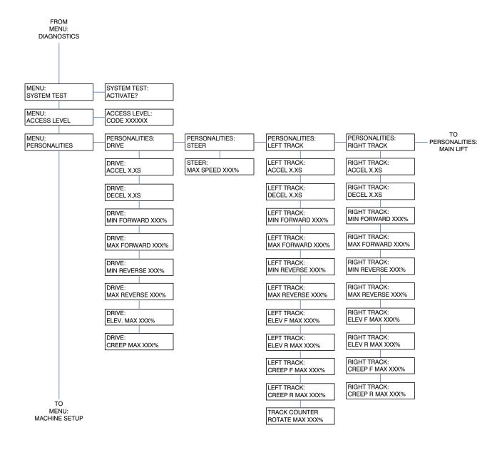
Figure 6-16. Analyzer Flow Chart, Version 6.X Software - Sheet 4of 6
