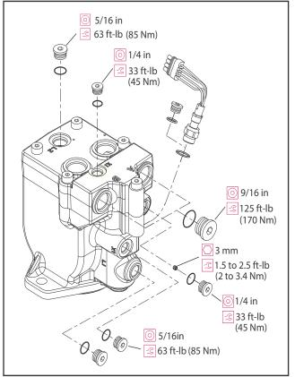
Figure 3-45. Plugs and Fittings Installation
