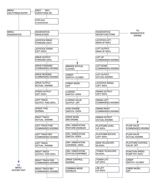
Figure 6-13. Analyzer Flow Chart, Version 6.X Software - Sheet 1of 6
