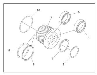
Figure 5-27. Cylinder Head Disassembly
