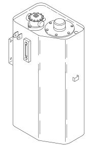
Lube Point(s) - Fill Cap Capacity - 27 gallons (102 liters); 23.6 gal. (89 liters) to the Full line on the sight gauge Lube - HO Interval - Check Level daily; Change every 2 years or 1200 hours of operation.
