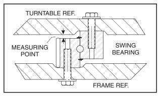
Figure 3-51. Swing Bearing Tolerance Measuring Point
