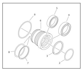
Figure 5-66. Cylinder Head Disassembly
