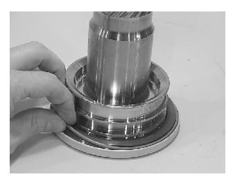
**4.** Using a seal tool install main pressure seal (205) on shaft (2) and end cap (4). Use seal tool in a circular motion.
