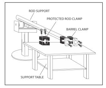
Figure 5-51. Cylinder Barrel Support
