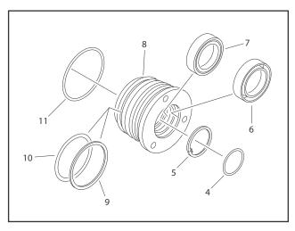
Figure 5-46. Cylinder Head Disassembly
