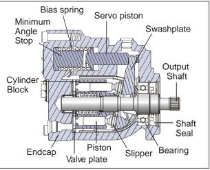
Figure 3-24. Drive Motor Cross Section
