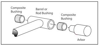
Figure 5-77. Composite Bushing Installation
