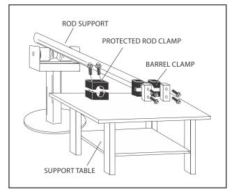
Figure 5-41. Cylinder Barrel Support
