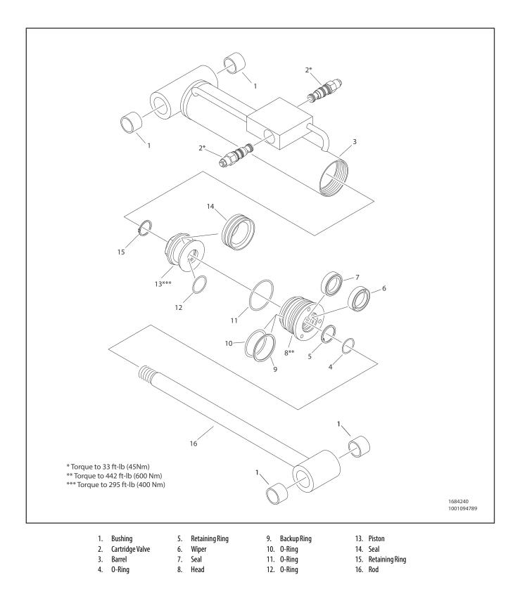
Figure 5-44. Platform Level (Slave) Cylinder
