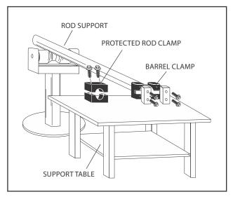
Figure 5-71. Cylinder Barrel Support
