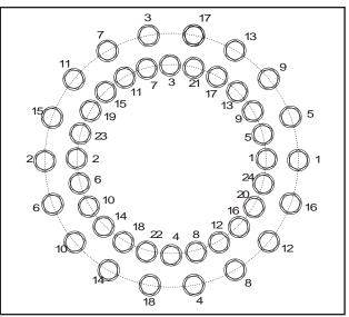
Figure 3-52. Swing Bearing Torque Sequence
