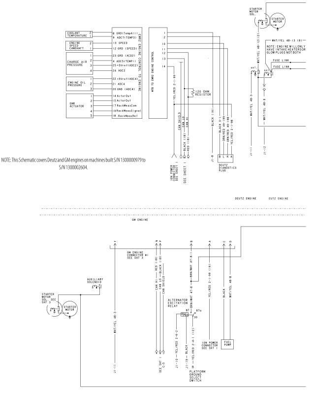
Figure 7-26. Electrical Schematic - Deutz EMR2 & GM Engine - Sheet 3 of 6
