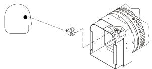
Every 500 hours of service, blow out the inside of the generator. If operating in a hostile environment, clean monthly.
