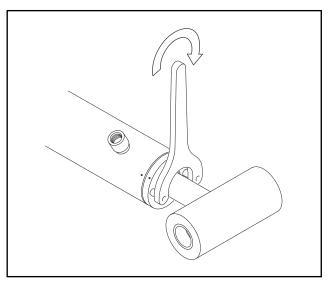
Figure 5-50. Cylinder Head Installation
