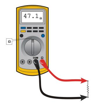
Figure 7-2. Resistance Measurement
