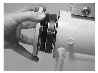
**11.** Before removing piston (3), mark housing (1) ring gear in relation to piston O.D. gear. There should now be timing marks on housing (1) ring gear, piston (3) and shaft (2).
