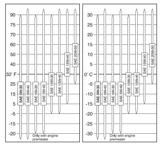
Figure 3-55. Engine Oil Viscosity
