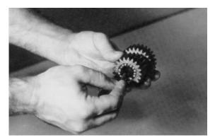
2. Place one spacer (3D) inside cluster gear (3F) so that it rests on top of the needle rollers.
