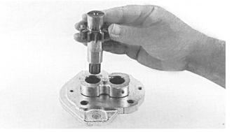
**12.** Remove drive shaft from mounting flange. There is no need to protect the shaft seal as it will be replaced as a new item.
