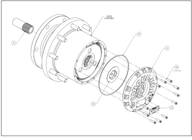
6. Cover10. Thrust Spacer19. O-ring9. Input Coupling14. Cover Bolts
