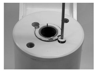
Using a 1/8" (3.18mm) drill bit, drill a hole in center of each lock pin to a depth of approximately 3/16" (4.76mm).
